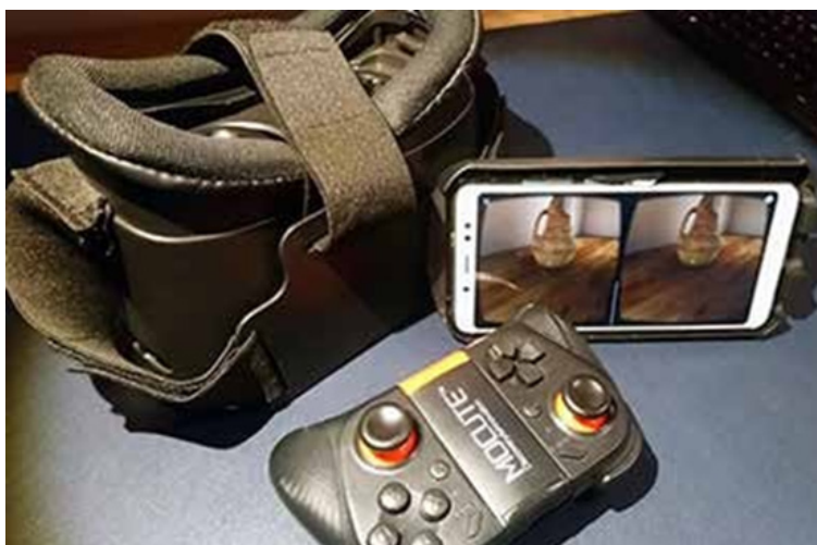
Figure 1. The test setup: VR frame, Bluetooth controller with a joystick, Android mobile device
